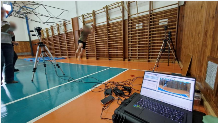
Hop trial: two tripod cameras, trigger cabling, live capture
