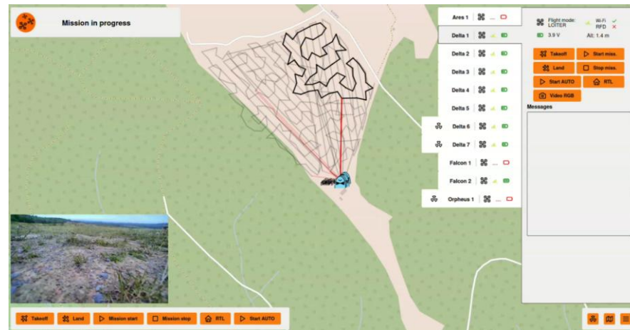
Command software: planned trajectories, live positions, telemetry and video of all assets
