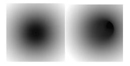
If we use certain image filters, we can extract a set of points (pixels of the image) highlighting a character of the tube in certain distance in front of the camera. These points (pixels) are using conic fitting algorithm to get conic (in this case our aim is to always get an ellipse) in IPNS representation (vector in R5,3  $\subset$  G5,3).
