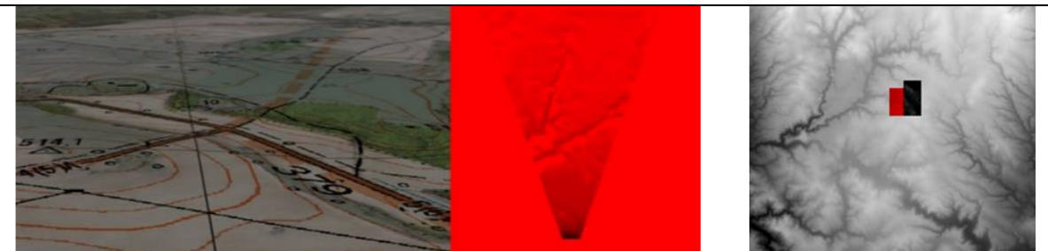
A depth map is obtained by reverse transformation, where the visual rendering transforms each individual map pixel, even with objects. This approach brings superior results, millions of pixels are calculated. (on the left) Parallel execution of Floating Horizon Algorithm on CUDA platform, solution performance is about 150 times faster, comparing to the modern CPU processor (average time 2832ms, observer source area 1x2Km, visibility destination area 1.4x 2.5Km, and terrain square resolution 5m.) (on the right)
